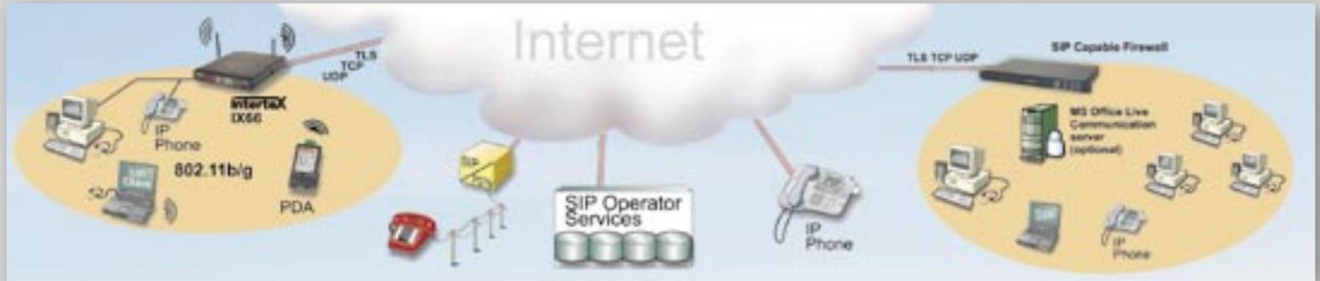
The IX66 is the first broadband router in the world to allow SIP communication. It has a very general and well-proven SIP support by integrating a SIP proxy and a SIP registrar, dynamically controlling the NAT and firewall. Conventional firewalls and NAT routers cannot even be configured to handle SIP between a LAN and the Internet!
