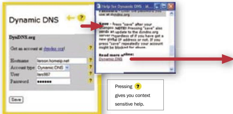
A dynamic DNS client allows your servers to be accessed by an Internet name (URL) instead of an IP number, even if you have not received a fixed IP address from your operator. It is very useful if you want to operate a WEB server or when using the IX66 as a SIP server.
