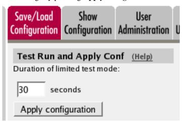
When the configuration has been applied, you should save a backup to file. Press **Save config to CLI file** to save the configuration.
